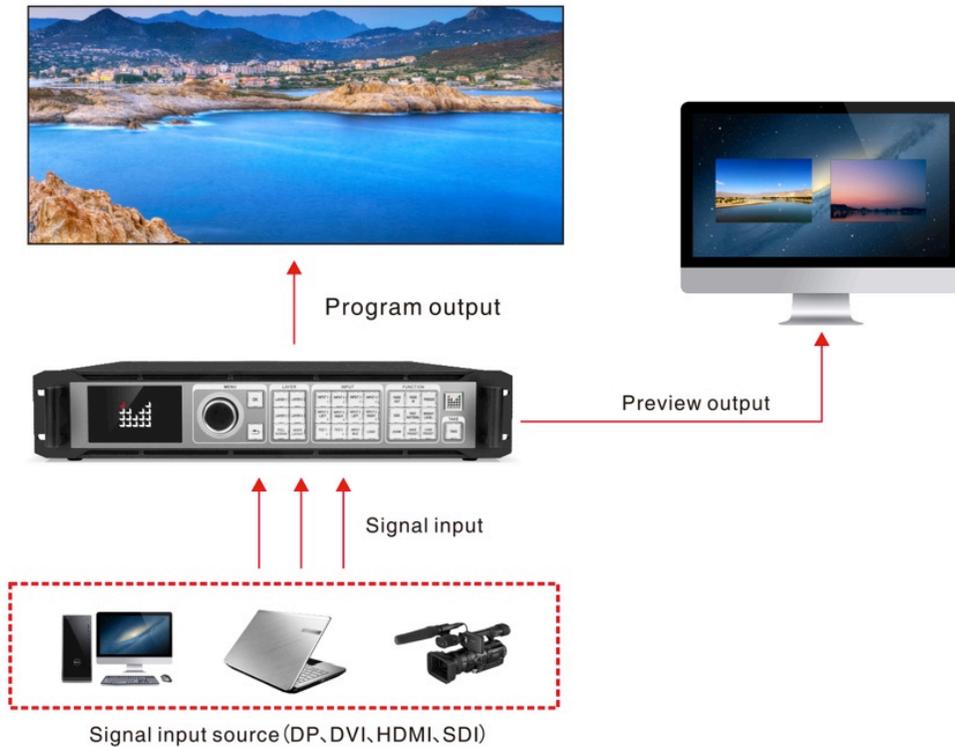
HDMI 1 is program output; HDMI 2 is preview, support fade switch among 3 images and 3 images. Under switcher mode, it only supports HDMI output.
