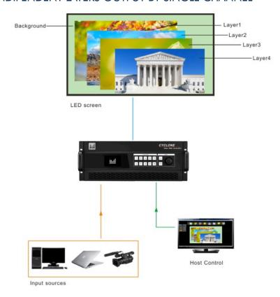
One DVI output channel is able to display 4 independent layers and one high definition background. The position, size and order of each layer can be set freely. Input source of any layer can also be set freely with the machine's inner video matrix.
