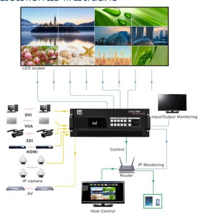
High resolution LED Wall splicing will be realized with corresponding sending cards and the machine's output customization. One 4U chassis machine supports 32 times splicing at most. One 3U chassis machine supports 16 times splicing at most. No frame drop and image tear. Supports 4Kx2K DP input and high resolution pixel-lopixel display.
