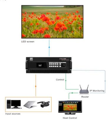
By connecting the network control port, the IP monitor and the host computer into one local area network, it is able to monitor all the input and output by the host software.
