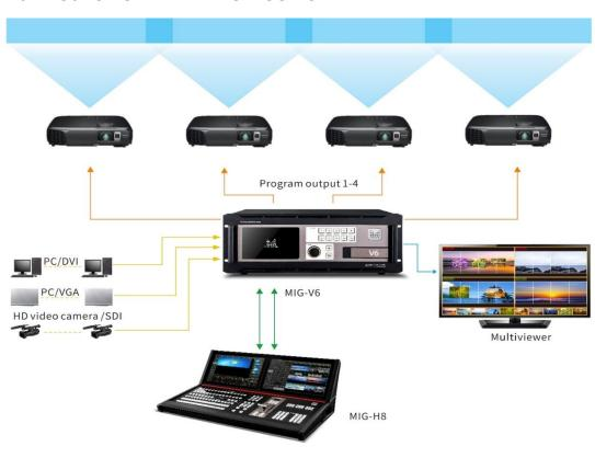
Each output port's blending size, position, blending direction, gamma rate can be set up separately, it's applicable for both program output and aux output; each V6 supports maximum 8 projectors for blending mosaic.
